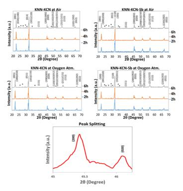
Figure 1. XRD patterns of KNN-KCN and KNN-KCN-Sb ceramics sintered at 1100 °C for 2, 4 and 6 h and in air or oxygen atmospheres with peak splitting at  $2\theta \approx 44.5$ -46.5°.
