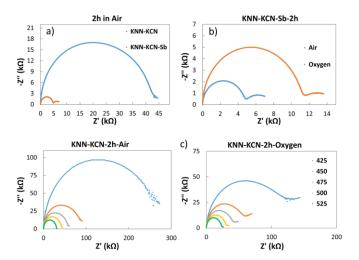
**Figure 4.** (a) 500 °C Z' vs Z" curves of KNN-KCN and KNN-KCN-Sb samples sintered in air for 2h (b) 500 °C Z' vs Z" curves of KNN-KCN-Sb samples sintered in air and oxygen atmosphere for 2h (c) Z' vs Z" curves of KNN-KCN samples sintered at different atmospheres as a function of measurement temperatures between 425 and 525°C.
