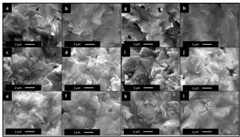
**Figure 2.** SEM images of KNN-KCN (a-b) 2h in air and oxygen atmosphere (c-d) 4h in air and oxygen atmosphere (e-f) 6h in air and oxygen atmosphere and KNN-KCN-Sb (g-h) 2h in air and oxygen atmosphere (i-j) 4h in air and oxygen atmosphere (k-l) 6h in air and oxygen atmosphere.
