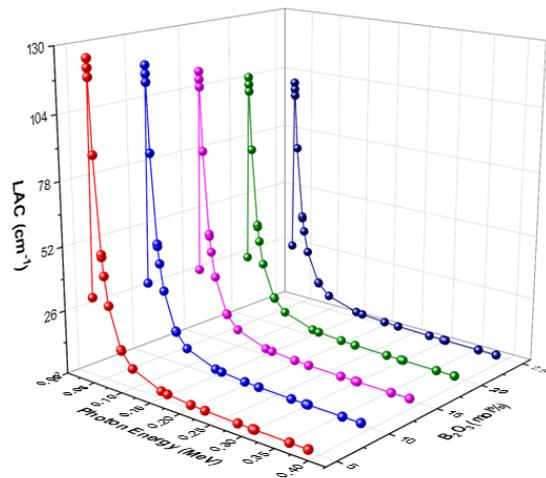
Figure 2. The findings for LAC values versus photon energies on the basis of the increasing  $B_2O_3$  doping rate.
