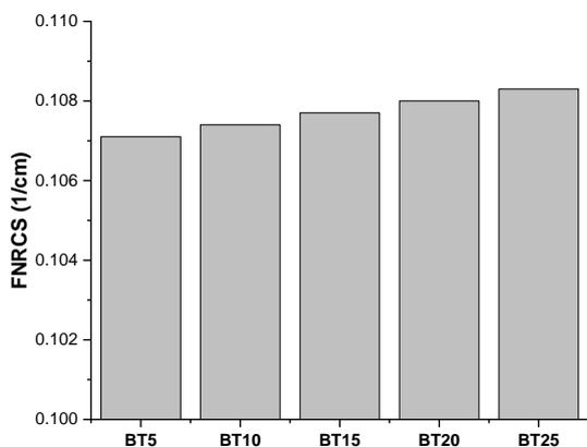
**Figure 3.** The findings of  $FNRCs$  for the BT5 to BT25 glass series.
